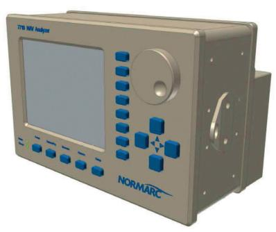
The NORMARC 7710 NAV Analyzer is used to adjust, verify and record parameters of ILS (Localizer, Glide Path, Marker Beacon) and VOR ground systems according to ICAO 8071. The NAV Analyzer's functionality substitutes instruments like ILS/VOR receivers, modulation meters and frequency counters. It incorporates all ILS and VOR channels selectable without any tuning or equipment changes. Facilitates measurement of
